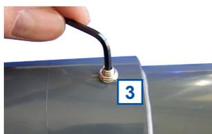
For cleaning or checking the reference measurement (function check) using the multifunctional slide, the spectrometer probe can be slid out of the probe carrier slightly after loosening of the hexagon socket.
