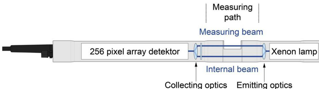
The central element of the emitter is a light source – a xenon flash lamp. This is complemented by an optical system to guide the light beam and an electronic control system to operate the lamp.
