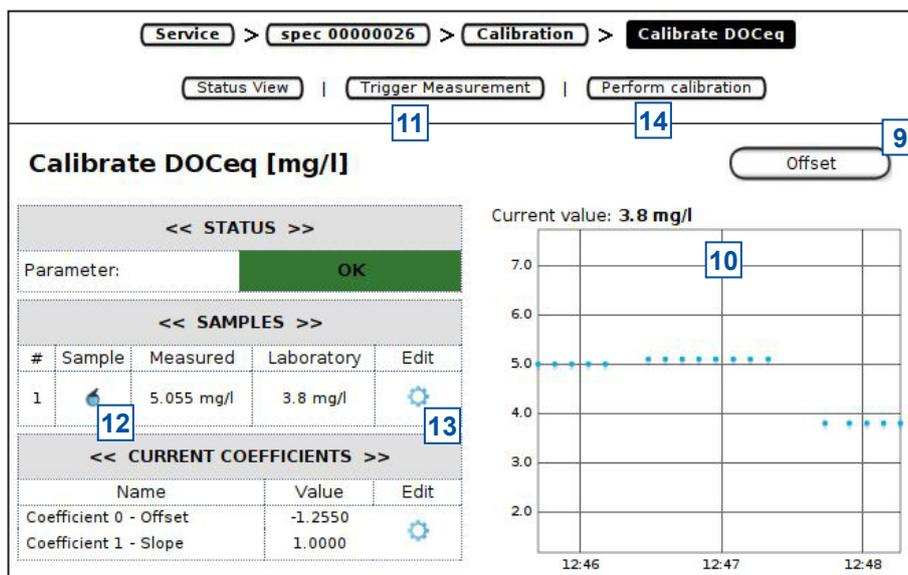
**12** Push the *Sample* icon to perform a new measurement and store the reading on the probe. Please note that the value (*Measured*) displayed below *SAMPLES* is the raw value, based on the global calibration. The *Sample #1* will be used for offset and linear calibration.
