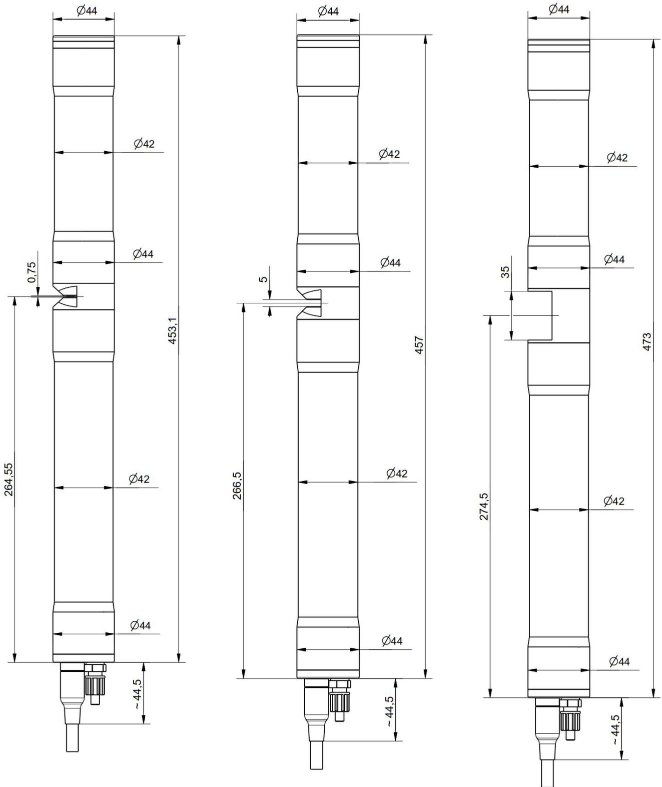
Dimensions of probe in mm:
