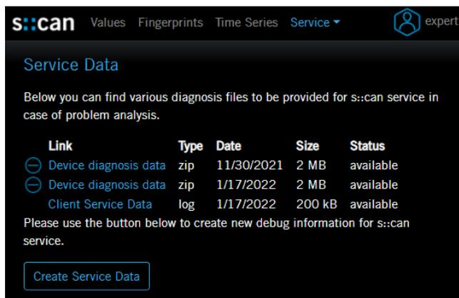
The service data can be created and downloaded directly in the Status display of monitor using the button *Sensor Diagnostics* (see figure on the right).
