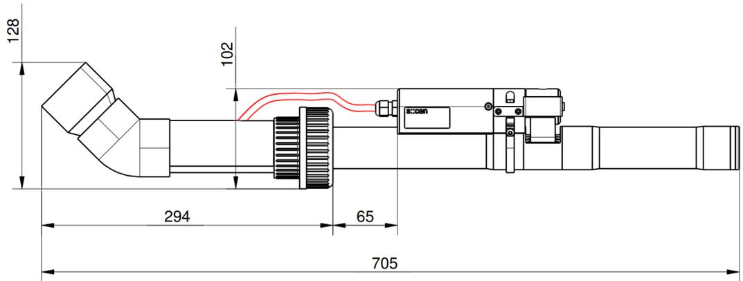
Dimension of probe carrier (F-140-V3) and required space for 35 mm spectrometer with ruck::sack in [mm]
