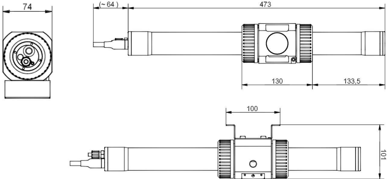
Dimension of flow cell (F-445-V3) and required space for 35 mm spectrometer probe in [mm]
