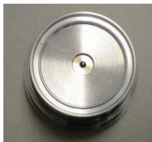
Figure 97: Remove the small o-ring
