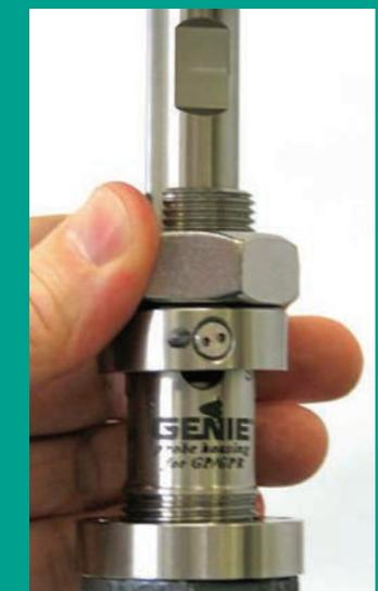
Figure 22: Tightening the insertion nut
