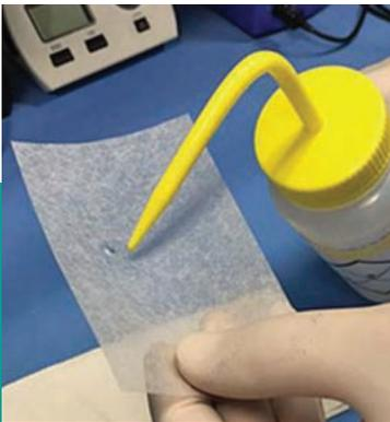
Figure 89: Applying acetone to lens tissue
