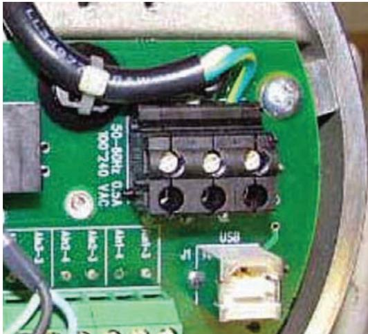
Figure 26: Power terminal block
