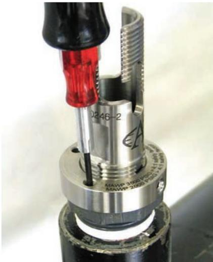
Figure 15: Tightening the Allen screws
