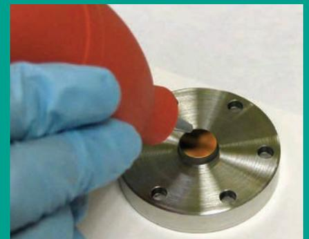
Figure 82: Blowing air onto the mirror
