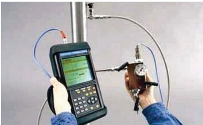
Figure 99: PM880 portable hygrometer
