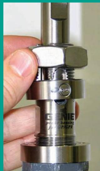
Figure 21: Loosening the insertion nut
