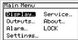
When the screen is unlocked, touch the *menu* key and the *main menu* appears with several options. To set up the display, select *display...* and press *enter*. The following screen appears:
