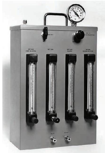
Figure 100: MG101 moisture generator
