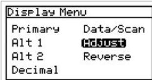
To modify the display contrast and brightness, from the *display menu* use the arrow keys to highlight *adjust* and press *enter*. The following screen appears.
