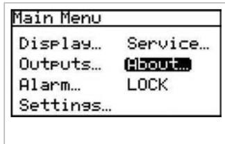
The calibration in use can be verified at any time using the **Aurora H2O about...** menu. From the *main menu*, select *about* and press *enter*. The following screen appears.
