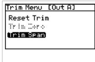
The *trim menu* returns with *trim span* highlighted. To change the span value, press *enter*. A screen similar to the following appears.
