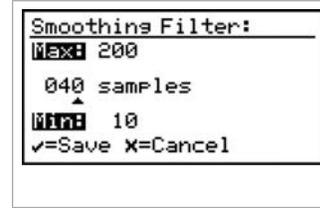
The smoothing filter setting is used to change the system responsiveness. It is a moving average filter to smooth the moisture readings. 1 sample = 1 scan. The minimum setting is 10 samples, or ~ 0.6 seconds. The maximum setting is 500 samples, or ~ 31 seconds. The default value of 40 samples, as set at the factory, is ~2.5 seconds.
