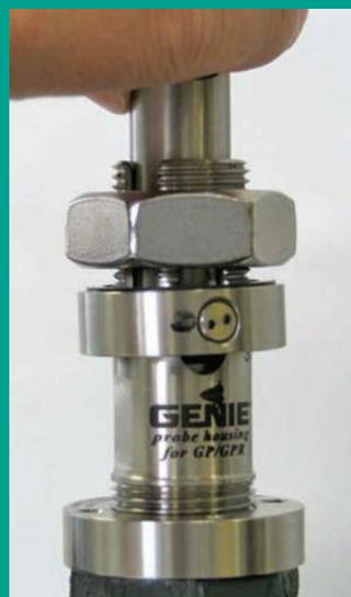
Figure 20: Rotating the probe
