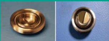
Figure 91: Replacing cleaned mirror into end cap assembly
