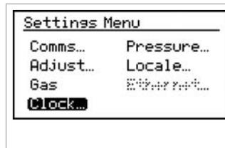
The clock settings are for informational purposes. They are used to keep track of the test analyzer start time and the laser operational time.
