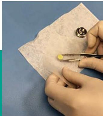
Figure 90: Cleaning a contaminated mirror
