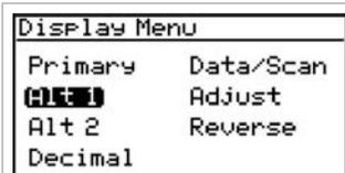
To set the units for *alt 1* and/or *alt 2*, use the arrow keys to highlight the one to be set, and press *enter*. The following screen appears:
