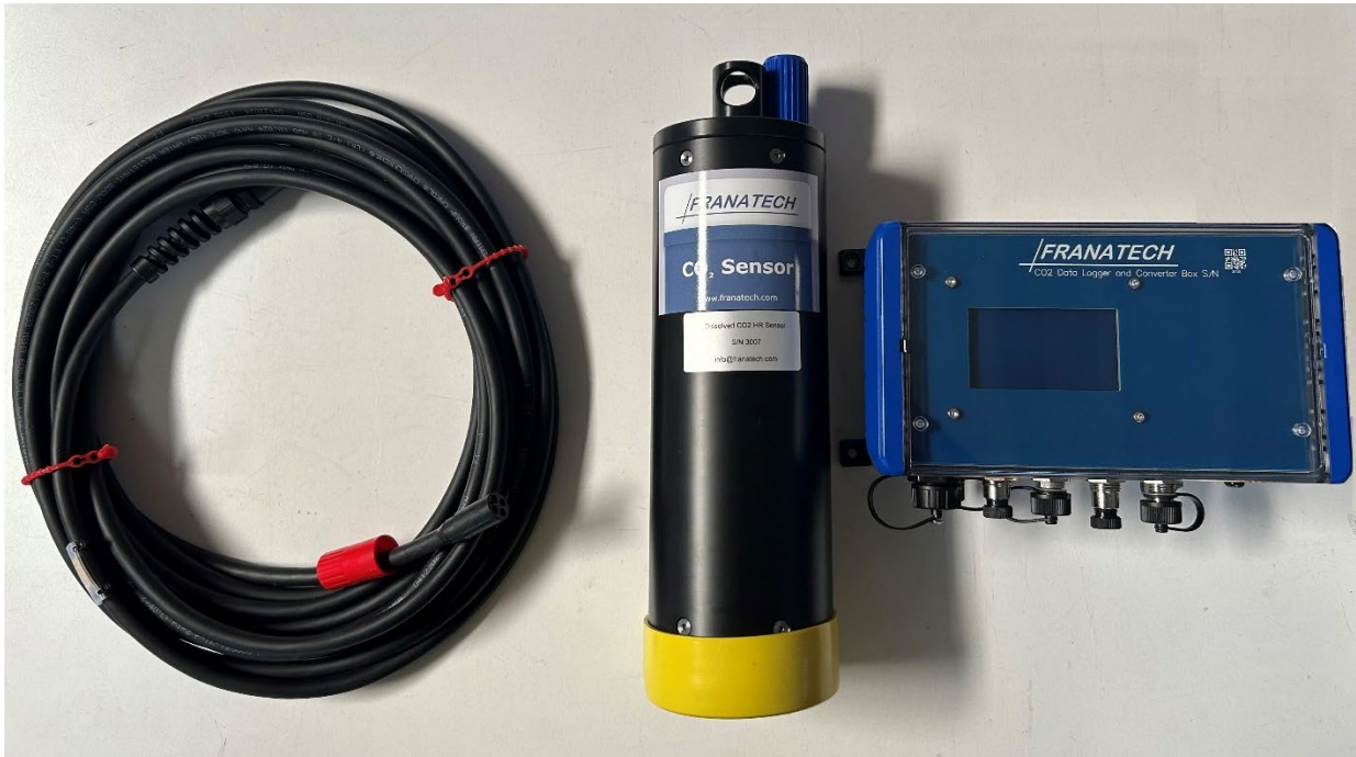
Sensor, Junction Cable, Junction Box
