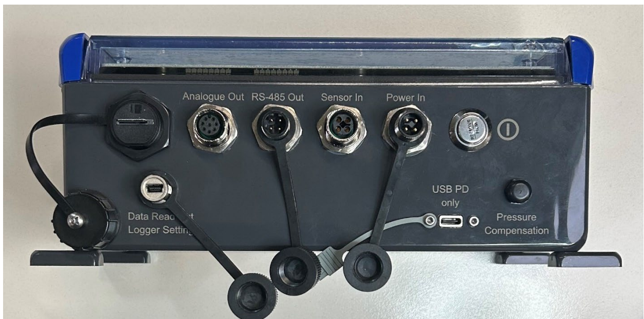
View of interface side of the Junction Box
