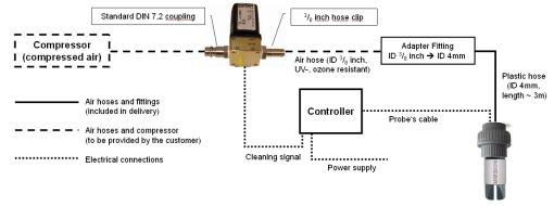
air supply is used in such a case the lowest maximum allowed pressure amongst those specified for the individual instruments is to be used to supply all instruments or the use of pressure reducing valves to supply each instrument with the correct pressure is necessary.
