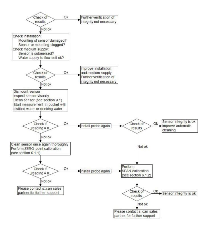
On a half year interval the zero point of the sensor should be checked in a medium free of suspended solids (e.g. distilled water or drinking water). If necessary a zero point calibration shall be performed (please refer to section 6.1.1).
