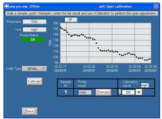
When selecting the calibration type <u>Default SPAN</u> and pushing the button <u>Calibrate!</u> the default slope (factory default) will be activated again.
