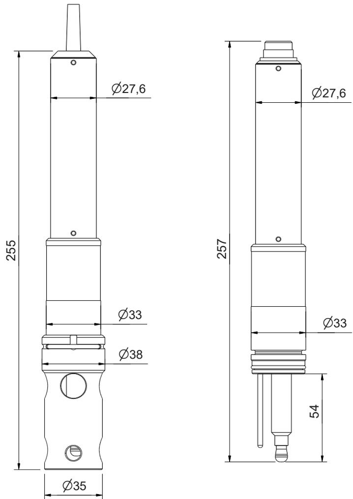
Dimensions of redo::lyser / pH::loyser cable version (left) and plug version (right)
