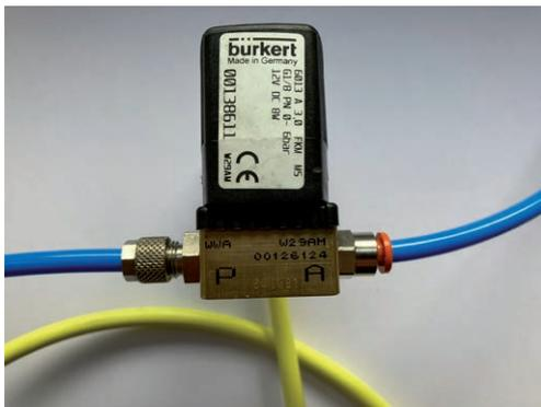
The adapter fitting of the pressure connection set (B-41) can be removed to connect the blue tube directly to the push-pull fitting of the cleaning valve. The same type of tube can be used to connect the cleaning valve to the s::can compressor.
