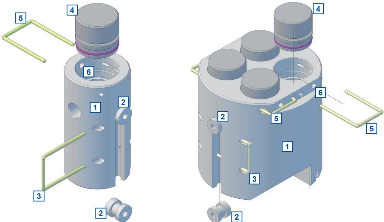
The flow cell itself [1] can be mounted directly on a solid and flat surface (wall, mounting panel, etc.) with the two fixing holders [2]. The position of the flow cell is secured by the mounting bracket [3] (see figures above).
