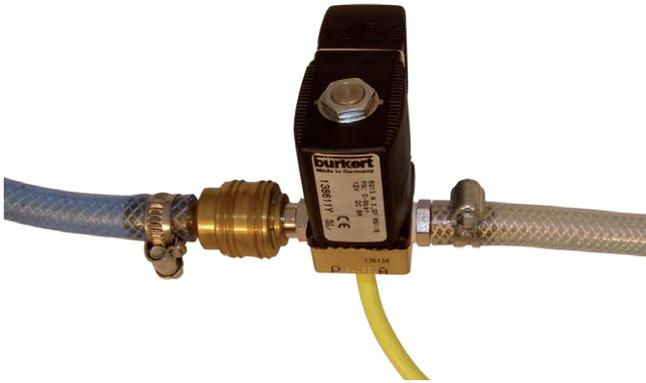
A compressed air hose (to be provided by customer, ID 8 to 9 mm) must be used to connect the adapter fitting of the pressure connection set (B-41) to the output side of the cleaning valve (marked with A). Fasten the air hose with hose clamps.
