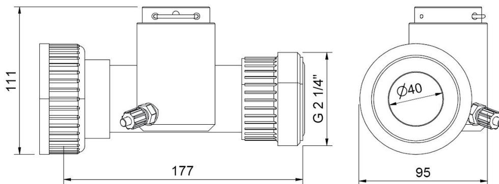
Dimensions of flow cell in mm (F-48-SENSOR)
