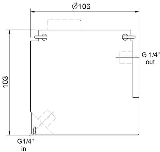
Dimensions of flow cell clean water for 4 sensors (F-45-FOUR) in mm
