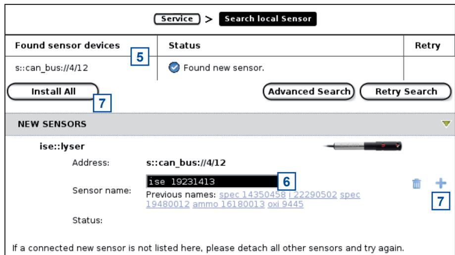
8 moni::tool will install the sensor and switch to the Service display. The new sensor is displayed in the system overview.
