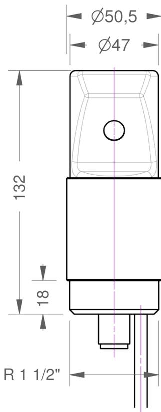
Dimensions of oxi::lyser in mm
