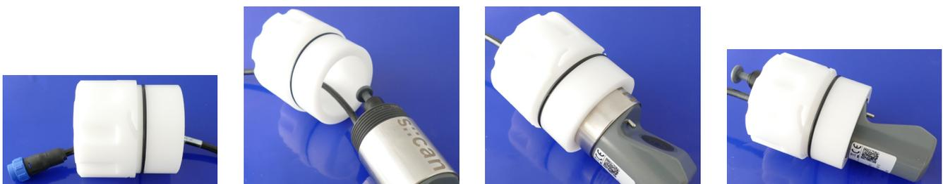
⚠ For easier handling put a little bit of grease onto the black o-rings. In case the flow cell will leak on top, the thread of the oxi::lyser can be wrapped around with some teflon strip before the sensor is screwed into the adapter.
