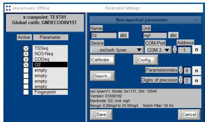
As soon as the sensor has been detected, information will be shown in the grey text field in the lower part of the dialogue window (model and serial number, version, electrode, unit, measuring range and filter settings).
