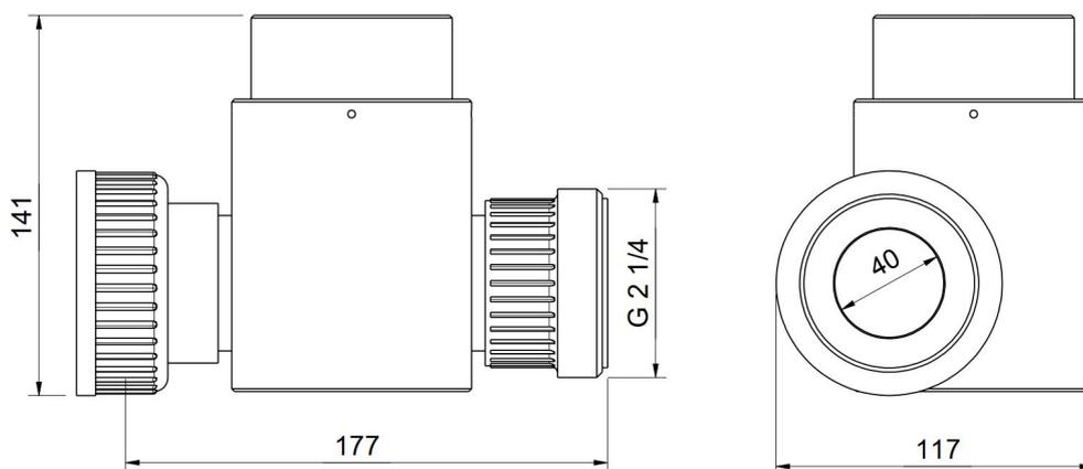
Dimension of flow cell setup in mm (F-48-OXI)
