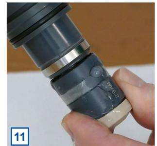
**12** Spill the excessive electrolyte from the sensor body with clean tap water or distilled water.
