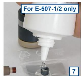
**8** Now move the bottle over the membrane cap without stopping the flow. Let the electrolyte flow slowly along the edge into the membrane cap up to the top. This procedure will avoid air bubbles within the electrolyte.
