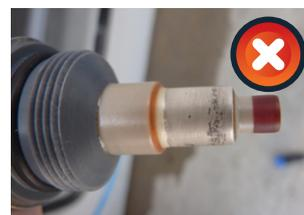
The electrolyte and membrane cap need to be replaced every 12 months or if the local calibration failed (see section 6). The replacement is performed by the following steps:
