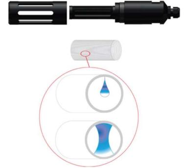
Excess water in the tubing can damage the pressure transducer if actual contact is made with the pressure sensitive wafer.
