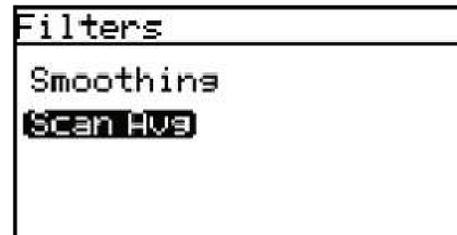
The Scan Average setting is used to change system noise rejection. By averaging entire scans, the Signal/Noise Ratio (SNR) can be increased. This is particularly useful in the presence of certain background gases, which can interfere with the moisture absorption peak, or introduce background noise.
