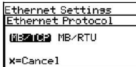
To use Modbus/TCP over Ethernet, the Ethernet module must also be configured as follows:
