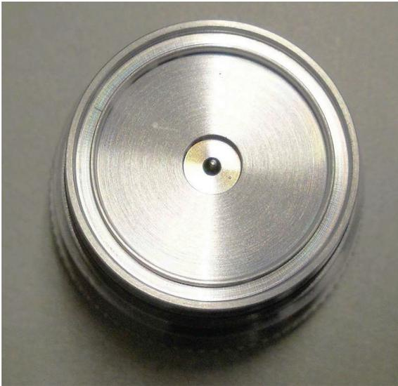
Figure 65: Remove the small O-ring
