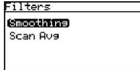
The Smoothing Filter setting is used to change the system responsiveness. It is a moving average filter to smooth the moisture readings. The minimum setting is 1 scan and the maximum setting is 501 scans. The default value of 128 scans, is set at the factory prior to shipment.
