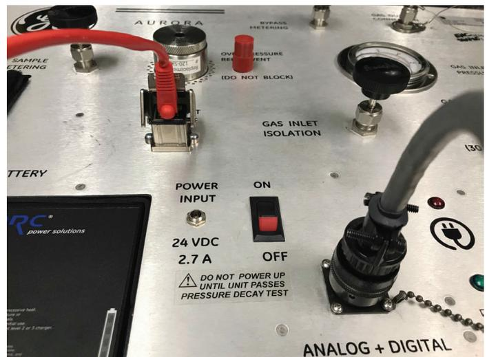
Figure 3: Aurora TransPort I/O cable connections
