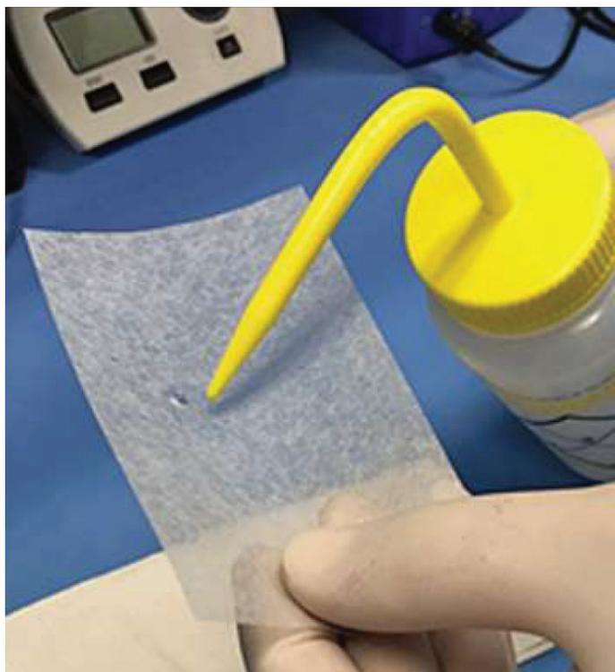
Figure 56: Applying acetone to lens tissue
