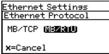
To use Modbus/RTU over Ethernet, the Ethernet module must also be configured as follows:
