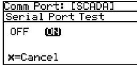
Enable Test mode by selecting ON and pressing **Enter**. The Aurora TransPort transmits SCADA waiting or SERVICE waiting (see *Figure 11* below), depending on the port being tested.
