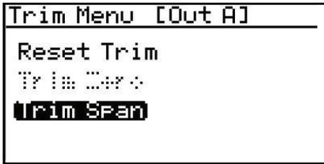
This will cause the Aurora TransPort to output 20.000 mA on the output being trimmed. The output value should then be read using the connected recorder, SCADA equipment, or DVM. Enter the value read from the connected equipment as the Span Trim value.
