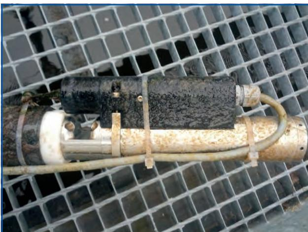
spectro::lyser with efficient automatic cleaning
