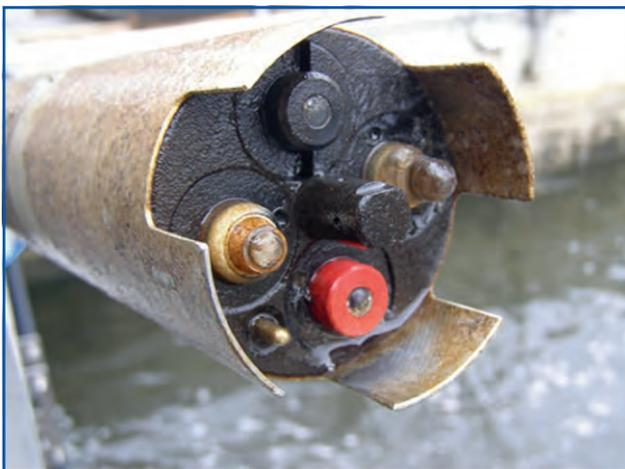
ammo::lyser in waste water effluent
