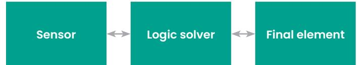
SIS automatically takes an industrial process to a safe state when specified conditions are violated. It permits a process to move forward in a safe manner when specified conditions allow.
