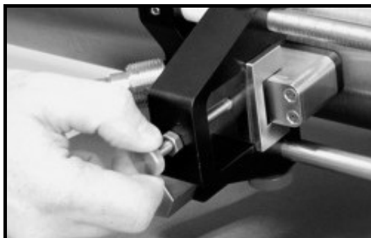
Figure 1-10: Installing the First Transducer
