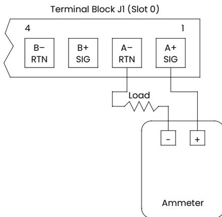
Figure 11: Ammeter connection (output A)
