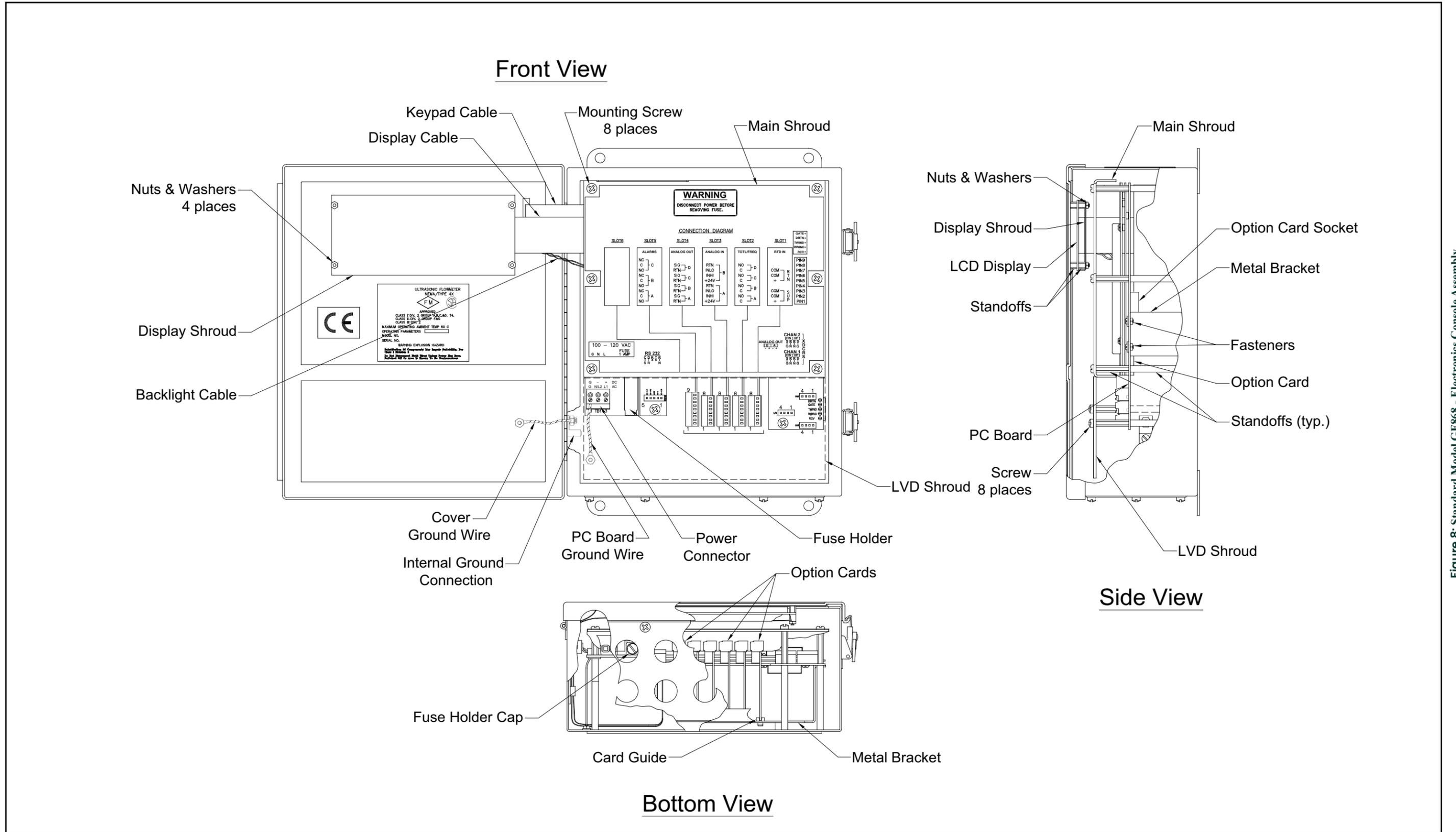
Figure 8: Standard Model GF868 - Electronics Console Assembly
