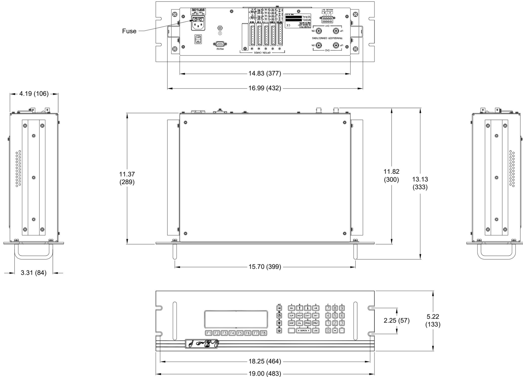
Figure 10: Model GF868 Rack Mount Enclosure Dimensions - (ref. dwg #712-1076)
