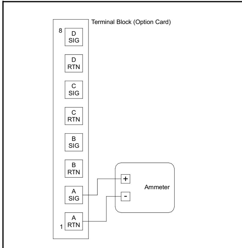
Figure 2: Ammeter Connection for Slots 1-6 (Output A)
