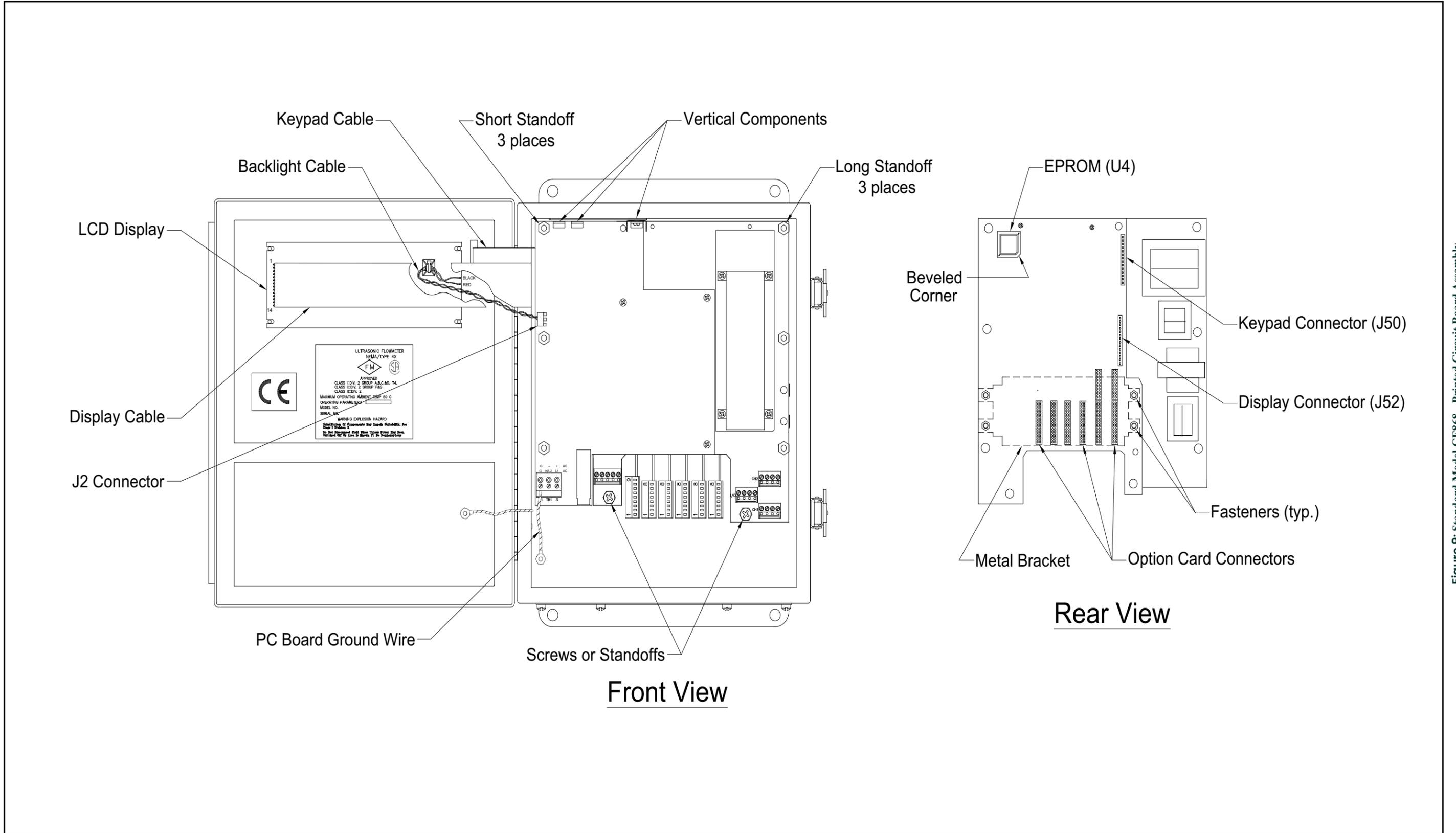
Figure 9: Standard Model GF868 - Printed Circuit Board Assembly
