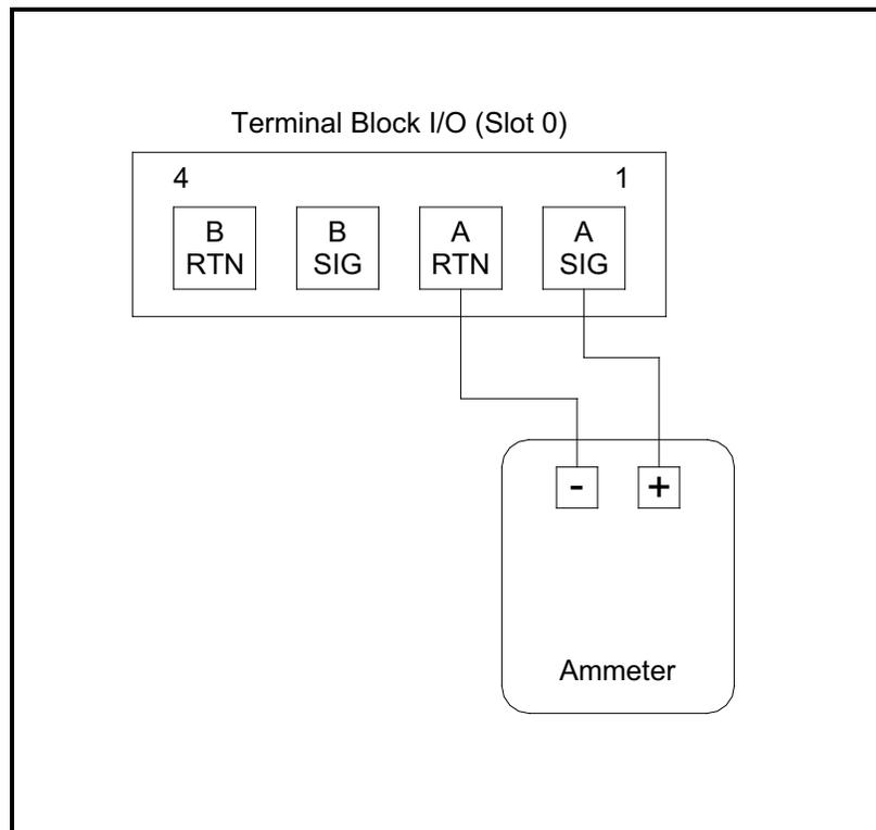
Figure 1: Ammeter Connection for Slot 0 (Output A)
