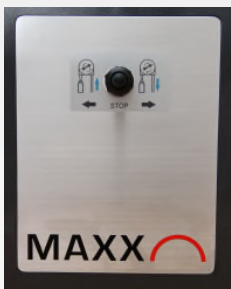
Fig. Control Switch for the Pump (Vacuum/Stop/Purge)
