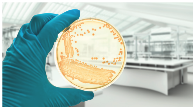
Fig. 1: Despite of the many disadvantages, heterotrophic plate count is still the standard methods for the quality control of drinking water.
