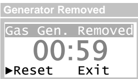
Figure 40. Generator Removed Display
