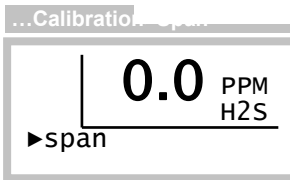
Figure 52 Sensor Span Cal. Setup
