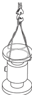
Figure 2: Sling-rigged lifting methods
