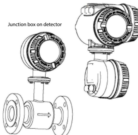
Figure 44: Remote mount amplifier
