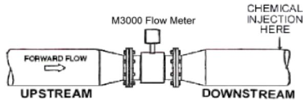
Figure 13: Meter installed upstream of chemical injection point
