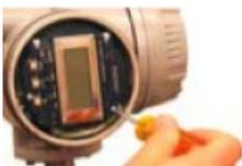
2. Remove the two display card screws and washers.
