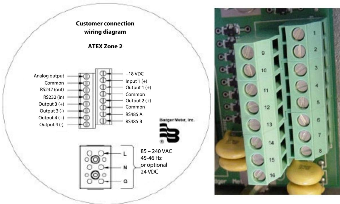
Figure 28: Amplifier output wire terminal block connections
