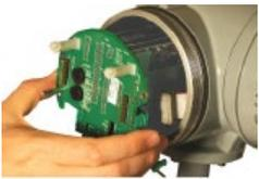
8. Gently remove the card stack from the amplifier housing. Do not tug or pull to remove the stack. Ease it out carefully.
