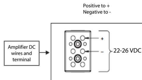
Figure 32: For 24V DC wiring
