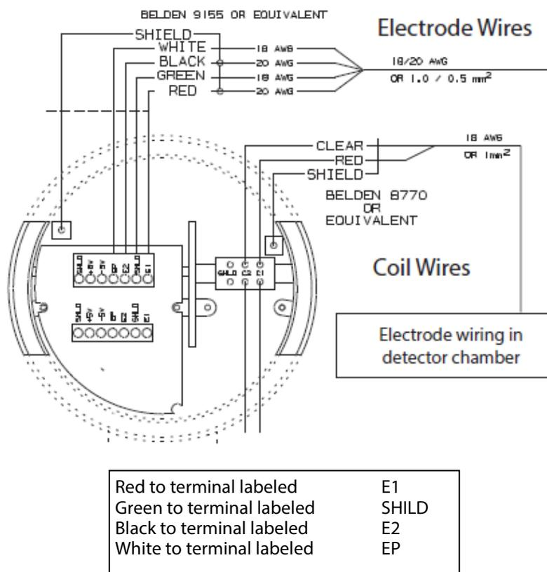
Figure 23: Electrode wiring in detector junction box
