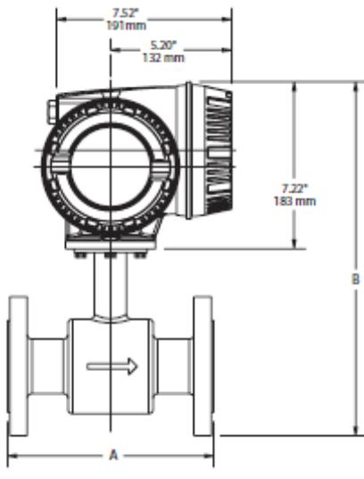
Figure 41: ModMAG® M3000 meter mount amplifier on detector
