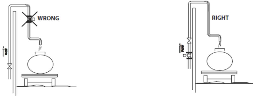
Do not install in a vertical, downward position.
