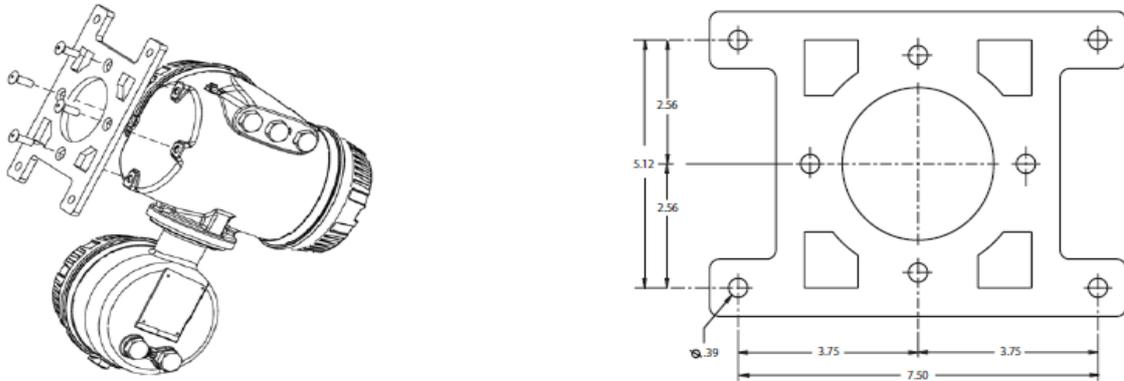
Figure 20: Mounting the bracket to the amplifier
