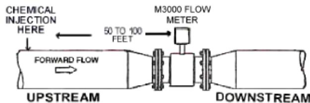
Figure 14: Meter installed downstream of chemical injection point
