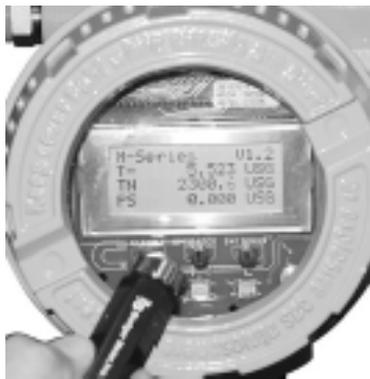
You can use a magnet wand to tap the + (plus), - (minus) and **E** switches. The amplifier display chamber cover stays on.
