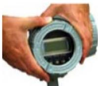
1. Remove display/programming chamber cover. Turn the cover counterclockwise to remove it from the amplifier. If necessary, use a strap wrench.
