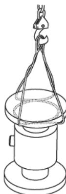
Figure 2: Sling-rigged lifting methods
