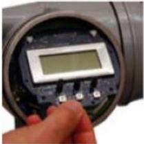
4. Gently pull card down and out from between the holding clips.
