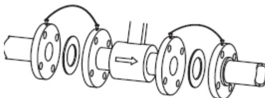
Figure 18: Conductive pipe grounding
