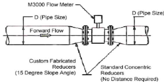
Figure 12: Pipe reducer requirements
