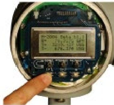
You can remove the display chamber cover and use your finger to tap the + (plus), - (minus) and **E** push buttons.
