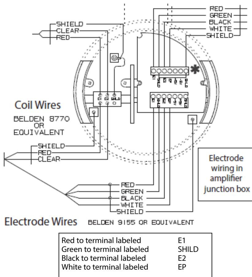
Figure 25: Electrode wiring in amplifier junction box
