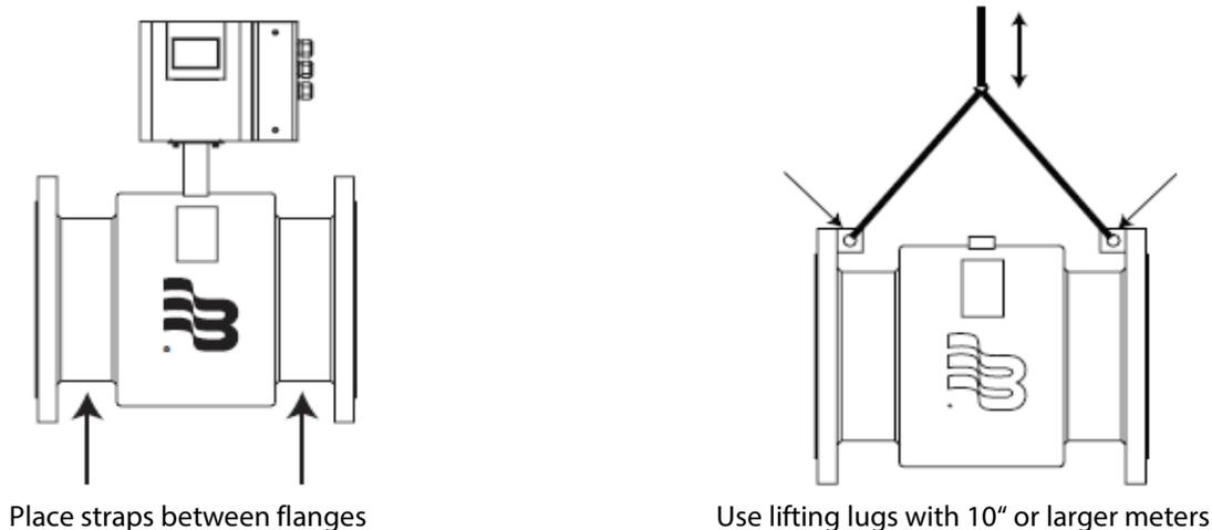
Figure 1: Rigging large units
