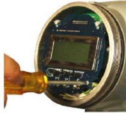
3. Tilt the card up and out approximately 45 degrees at the holding clips.
