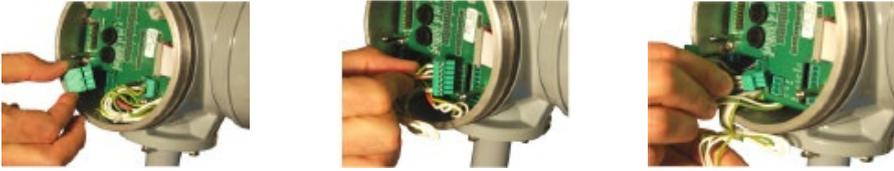
6. Disconnect the power, coil, electrode and I/O plugs and harnesses from the PCB interconnect card.
