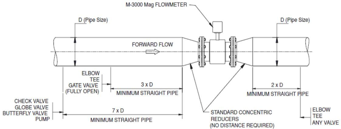
Figure 11: Minimum piping requirement
