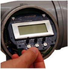
4. Fuses are in the round/black fuse holders. Use a flat screw-driver to turn the holder cap counterclockwise until the lock tab reaches the opening and the holder and fuse disengage.
