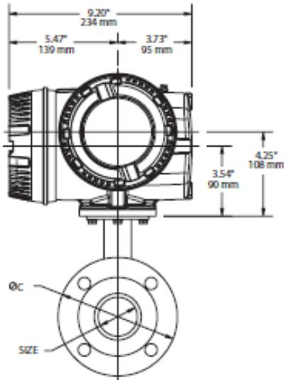
Figure 42: ModMAG® M3000 remote mount junction box on detector
