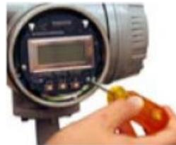
3. Tilt card up and out approximately 45 degrees at the holding clips.
