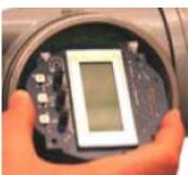
3. Tilt the card up and out approximately 45 degrees at the holding clips.
