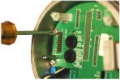
7. Remove the 4 screws holding the PCB stack in the amplifier housing. Place in storage for reuse.
