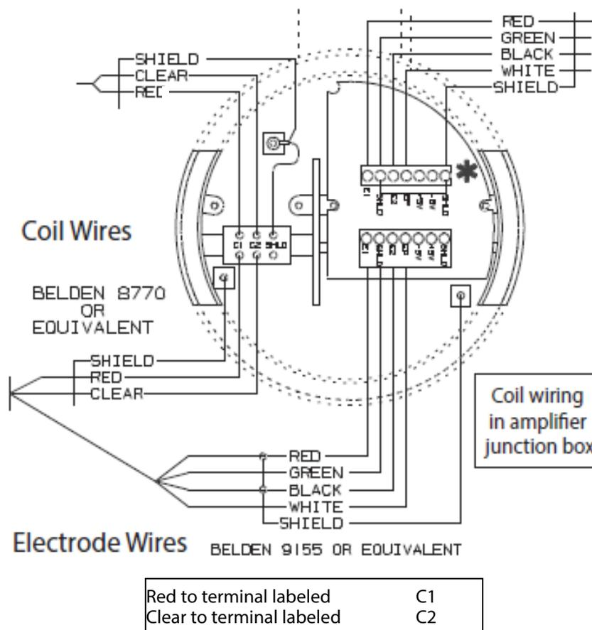
Figure 27: Coil wiring in amplifier junction box
