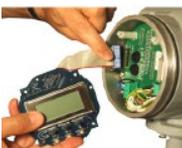
4. Gently pull card down and out from between holding clips.
