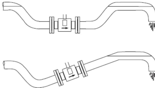
Figure 17: Pipe positioned to keep water in detector
