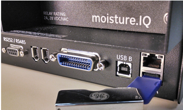
Figure 92: USB flash drive plugged into rear of chassis
