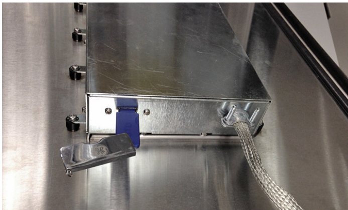
Figure 93: USB flash drive plugged into chassis inside the door
