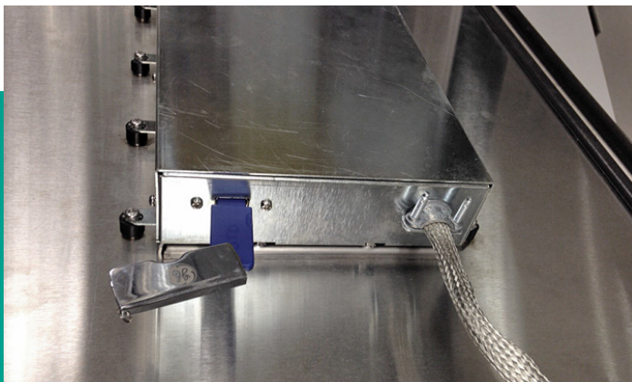
Figure 86: USB flash drive plugged into chassis inside the door
