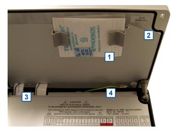
Used desiccant packages can be regenerated using normal drying processes (e.g. drying chamber at max 60°C or nitrogen). In this context, care must be taken that the cartridges cool down and are stored in an absolutely dry environment after the drying process.
