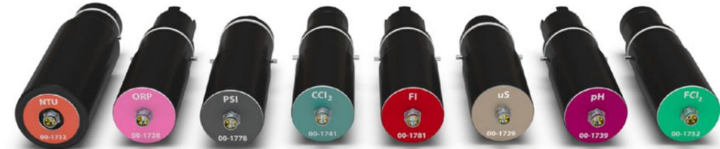
M-Nodes are complete water quality monitors equivalent to traditional online instruments, connected to the water supply using a purpose designed 'click-connect' flow cell arrangement. M-Nodes are connected in series to minimise water usage and can run at pressures up to 6 bar. Their ultra low powered nature means they have the ability to run autonomously for years at a time on small batteries. Alternatively they can be powered from a local plc or telemetry system.
