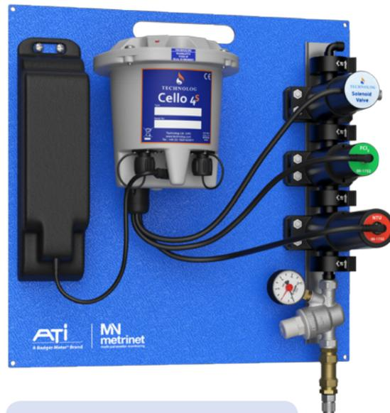
Example shown is a battery powered system measuring free chlorine and turbidity water quality parameters. Using a Technolog Cello 4s RTU with solenoid valve to save water by controlling the intermittent flow and connected to the distribution network via a PRV.
