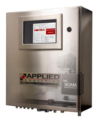
The OMA-300-InGaAs Process Analyzer produces results in real time by measuring the light absorbance of a liquid or gas sample by utilizing the Beer-Lambert law to correlate the light data to the chemical concentration of an analyte. The OMA-300-InGaAs uses an Indium Gallium Arsenide detector and can be configured to scan across in one of three wavelength ranges – 1350-1650nm, 1550-1850nm, & 1750-2150nm.
