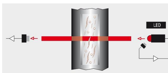
Figure 1: Measuring principle of the RET-5501
